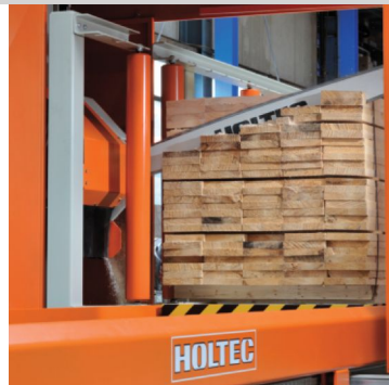
Variable cutting angle of 0 to 15° for optimal distribution of the cutting forces
